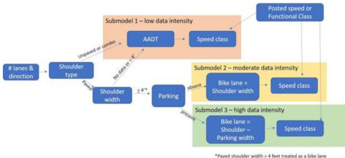
**Figure 2. Chart. Conceptual model illustrating the decision framework for calculating BLTS based on the presence and values of roadway attributes.**
