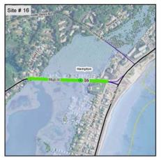
NH 27 (High Street), Hampton (Site 16): High Street is inundated between Mill Pond Lane and Kings Highway where the roadway passes through the Meadow Pond marsh/wetland area. The data indicates that flooding along this section of High Street would be widespread and impact all of the residential units on that segment as well as some of those that border Kings Highway such as along Gentian Road, Greene Street, and Meadow Pond Road.
