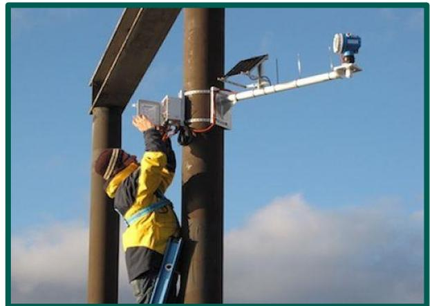
A state-of-the-art tide gauge is installed at the Hampton Fire Rescue Pier on Hampton Harbor by scientists from UMASS Boston, center for Coastal Environmental Sensing Networks (CESN) (Source - Coastal Adaption Workgroup [CAW])
