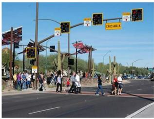
Figure 16: Pedestrian Hybrid Beacon (PHB) (Source: FHWA)
