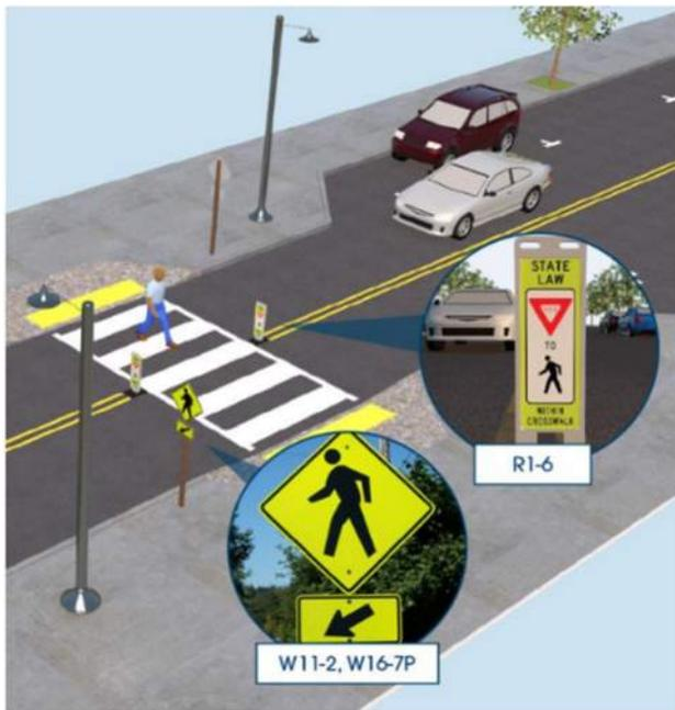
Figure 15: Crosswalk Visibility Enhancements (Source: FHWA)
