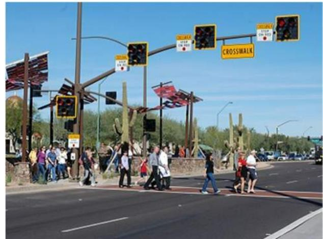
Figure 16: Pedestrian Hybrid Beacon (PHB) (Source: FHWA)
