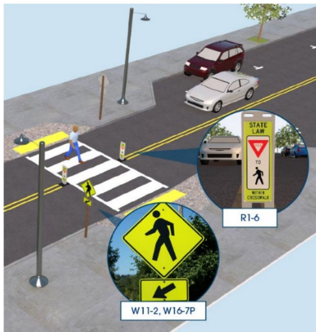
Figure 16: Crosswalk Visibility Enhancements (Source: FHWA)
